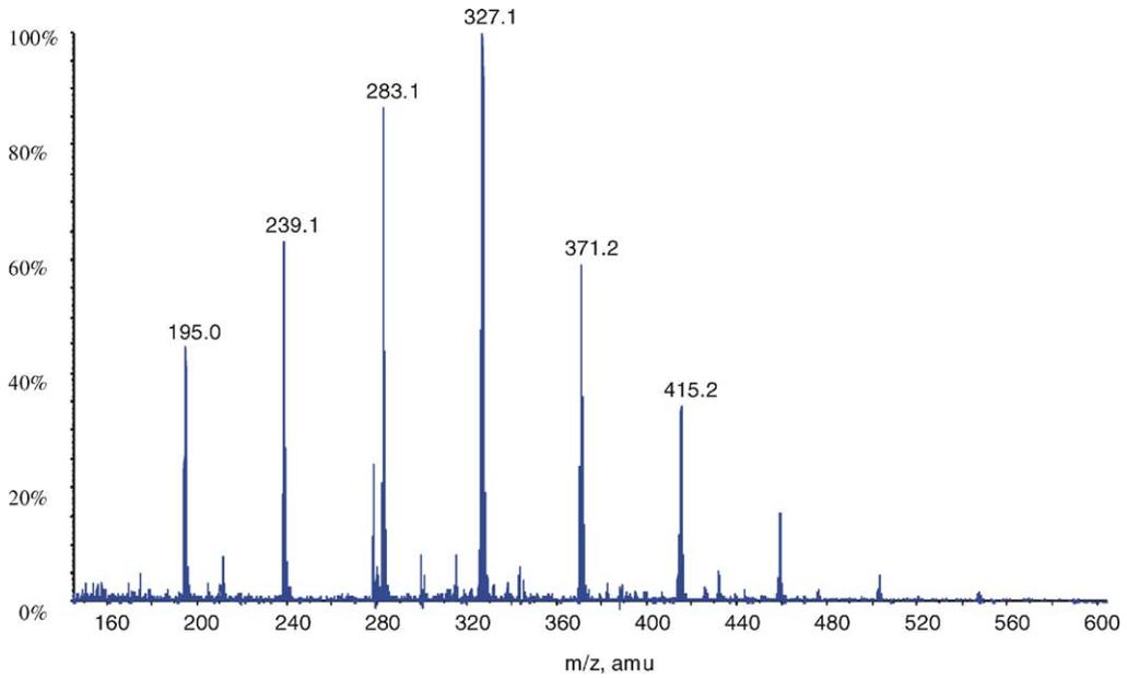
Fig. 1. Full scan mass spectrum of PEG 300 (from APCI).
